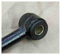
Now, no amount of pressure will make these new bushings as small as the originals. So, reinstalling them can be a bit of a chore. The end that
