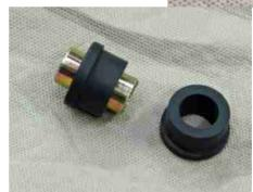
Now, I found that it helped to spray some Silicone lubricant in the holes at the ends of the strut rods – it makes it easier to slip the rubber bushing into the hole. I inserted one half of the bushing, then
